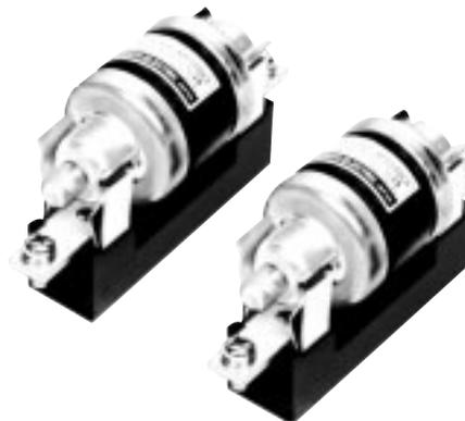
ZNR Transient/Surge Absorber, Type P is a suitable device to protect various electric equipment and semiconductive devices from instantaneous over-voltages like switching surges and induced lightnings. The Type P is characterized by the unique construction of plug-in type with a deterioration indicator.
